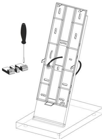
Connect the terminals to the previously installed cable. The terminals are located at the back of the indoor station.
