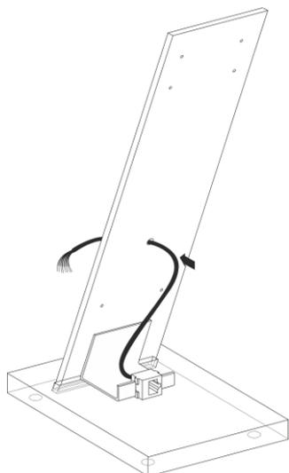
The connection adapter is located on the back of the table installation kit.
