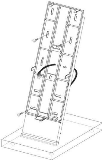
Using the screws attach the supporting frame of the indoor station to the table installation kit. Please use the fastening holes provided on the upper and lower part on the table installation kit.
