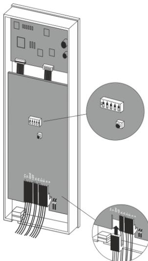
Set the SKS bus call address at the DIP switch on the back of the indoor station. Each address is assigned to a bell button at the door station. The SKS bus table of call addresses can be found in the appendix.
