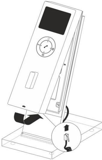
Remount the indoor station in the upper part of the supporting frame.
