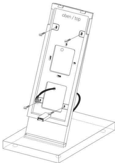
Using the screws attach the supporting frame of the indoor station to the table installation kit. Please use the fastening holes provided on the upper and under part on the table installation kit.
