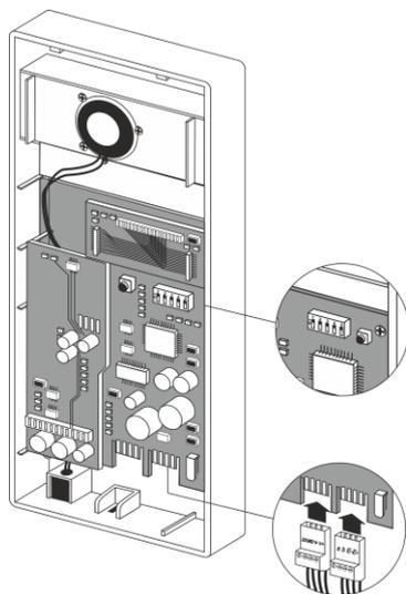
Set the SKS bus call address at the DIP switch on the back of the indoor station. Each address is assigned to a bell button at the door station. The SKS bus table of call addresses can be found in the appendix.
