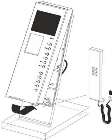
Remount the indoor station in the upper part of the supporting frame.
