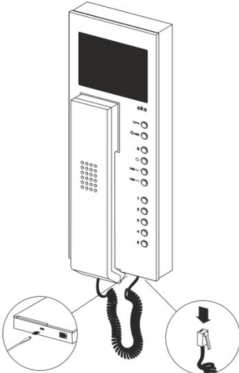
Use a screwdriver to release the indoor station from its supporting frame. This is done by inserting the screwdriver into the release opening at the bottom of the indoor station.
