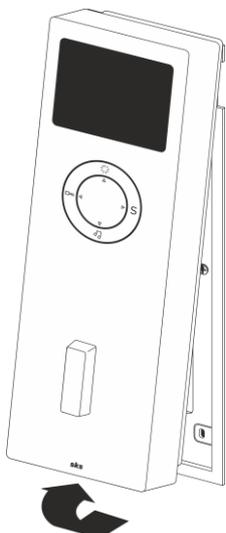
Carefully remove the indoor station from the support frame as shown in the drawing.
