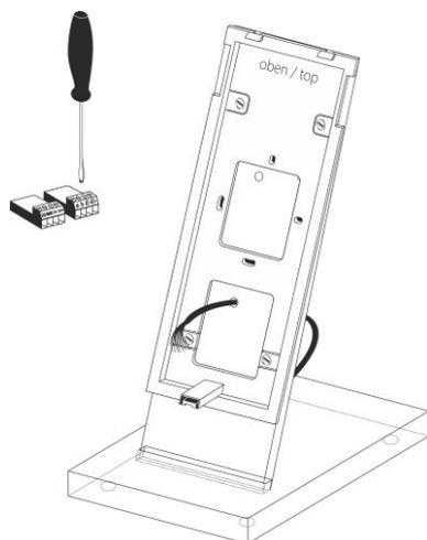
Connect the terminals to the previously installed cable. The terminals are located at the back of the indoor station.
